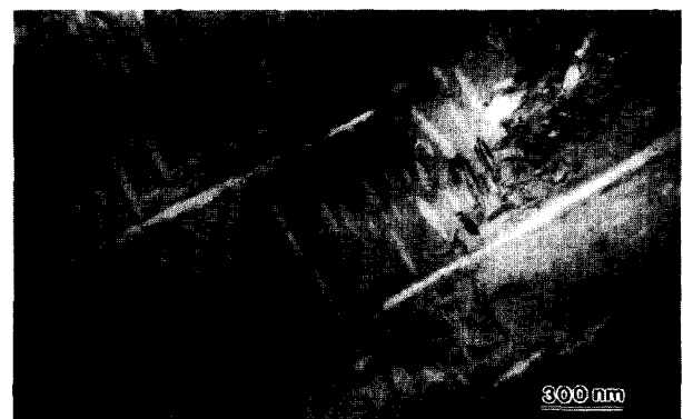
Fig. 5. Microstructure of sample aged at 1100°C for 145 h.
